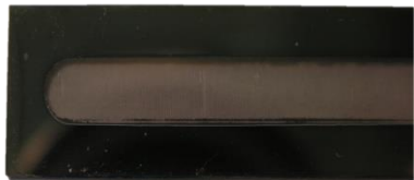
MMD: 1024 strips, 60 \mu\text{m} pitch, 40 \mu\text{m} width, 1,5 \mu\text{m} thick
