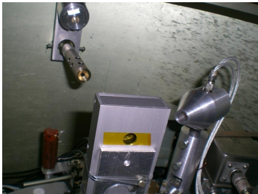
Spatial (Horizontal and Vertical) Proton Beam Profiles
