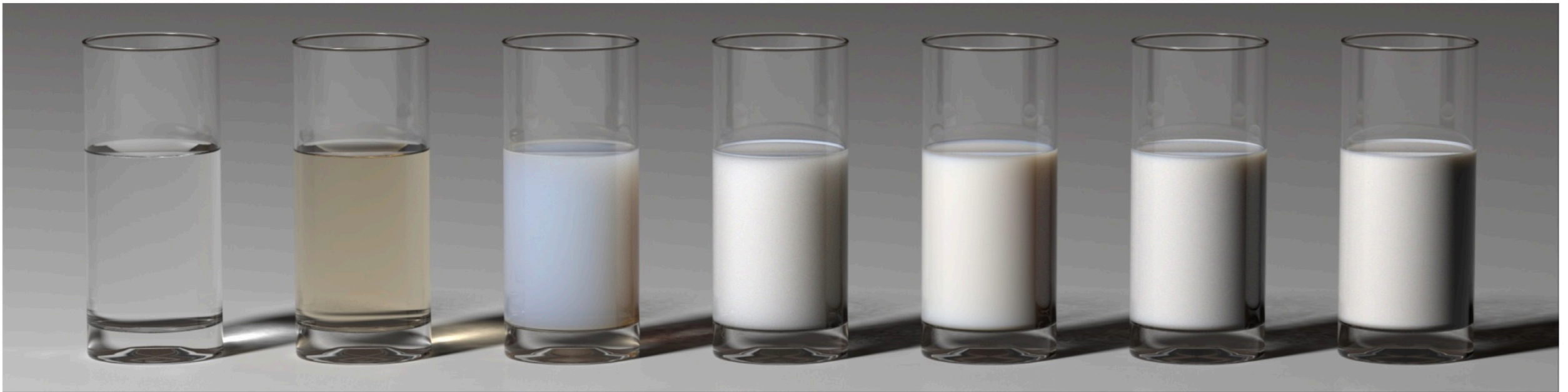
Figure 1: Rendered images of the components in milk as well as mixed concentrations. The optical properties of the components and the milk have been computed using the generalization of the Lorenz-Mie theory presented in this paper. From left to right the glasses contain: Water, water and vitamin B2, water and protein, water and fat, skimmed milk, regular milk, and whole milk.
