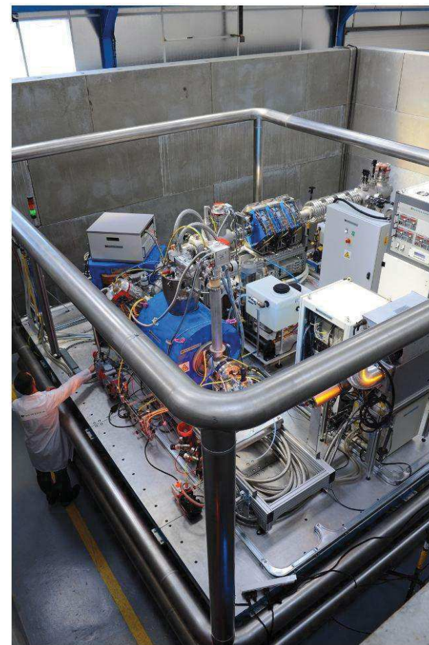
ECR source bench (Pantechnik / BARC, India) Magnetic elements SIGMAPHI
