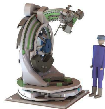
CEA: diffractometer to study nanostructures growth
