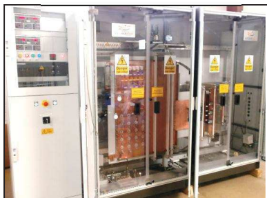
CRYRING Kicker magnet and pulser 3500A, 200 ns
