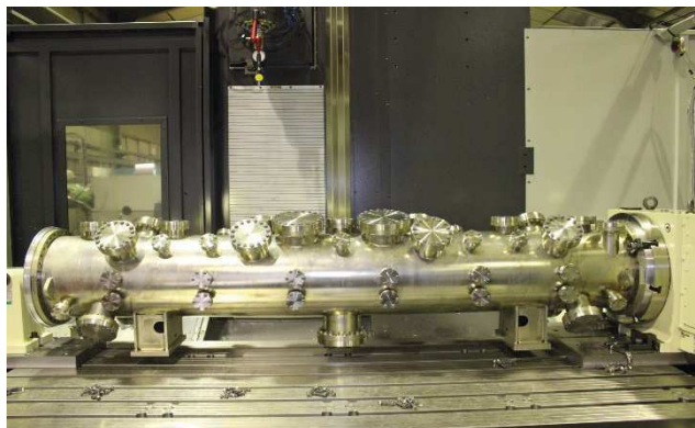
Vacuum chamber in the course of manufacturing (Synchrotron SOLEIL)
