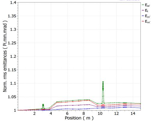
The three panels show the change of emittance in the three planes along the MEBT-3 for three different beam currents (4 mA, 3 mA, and 2 mA). Red and blue lines correspond to transverse emittances – horizontal and vertical, respectfully. Green lines correspond to longitudinal emittance.
