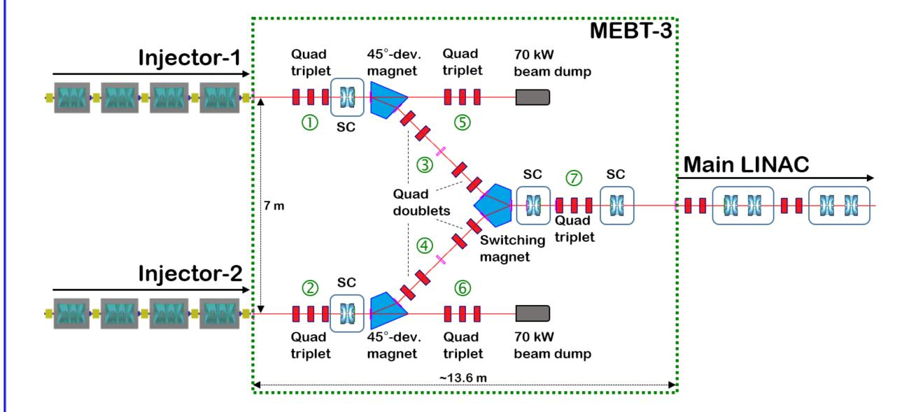
The MEBT-3 section between the two injectors and the main LINAC (dashed green line). It is divided into seven parts separated by two 45°-deviation magnets and a switching dipole connecting the two injectors to the LINAC section.
