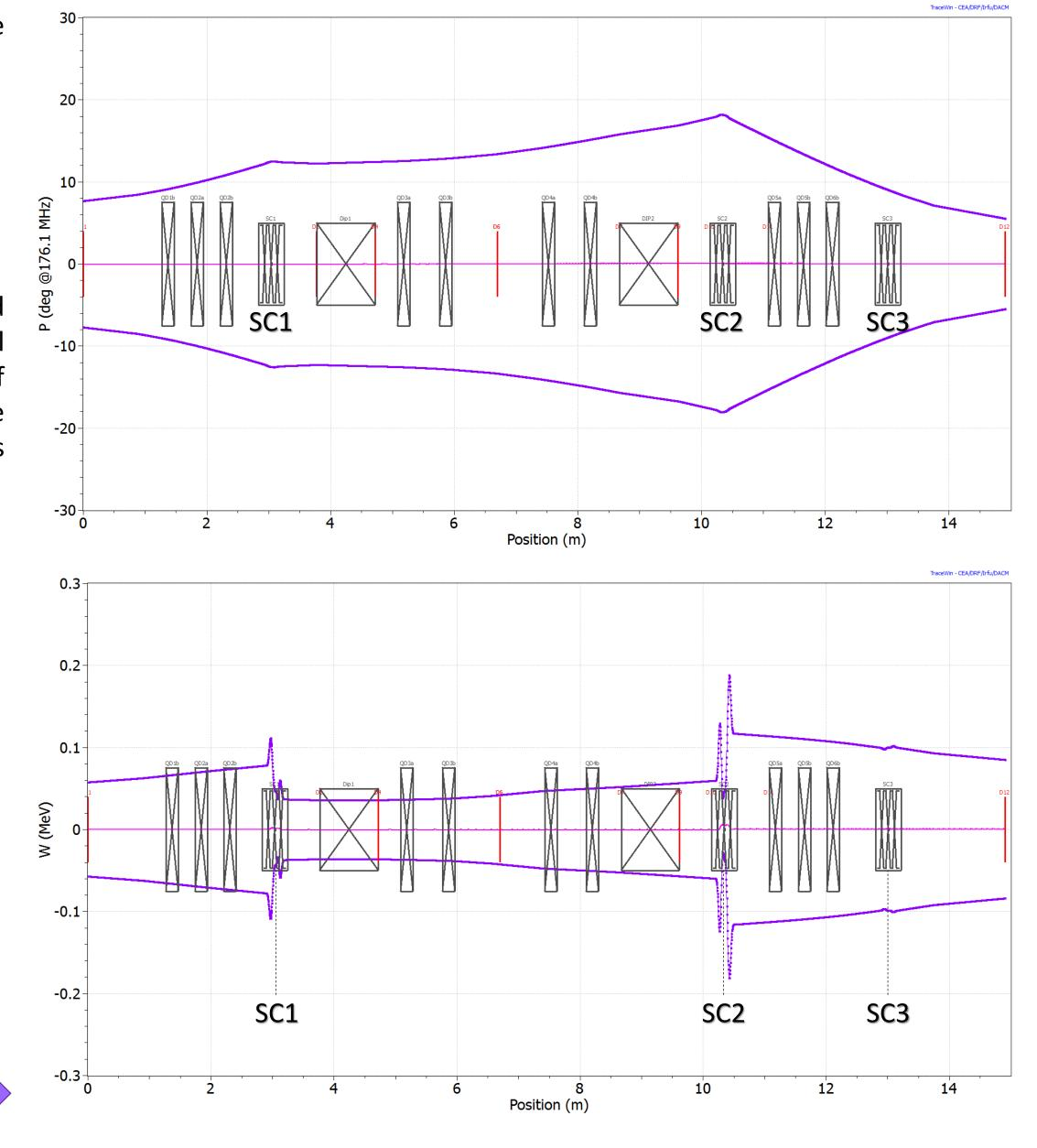
Longitudinal  $\pm 3\sigma$  envelopes along the MEBT-3 section. The phase and the energy spread are shown in the top and the bottom panels respectfully.
