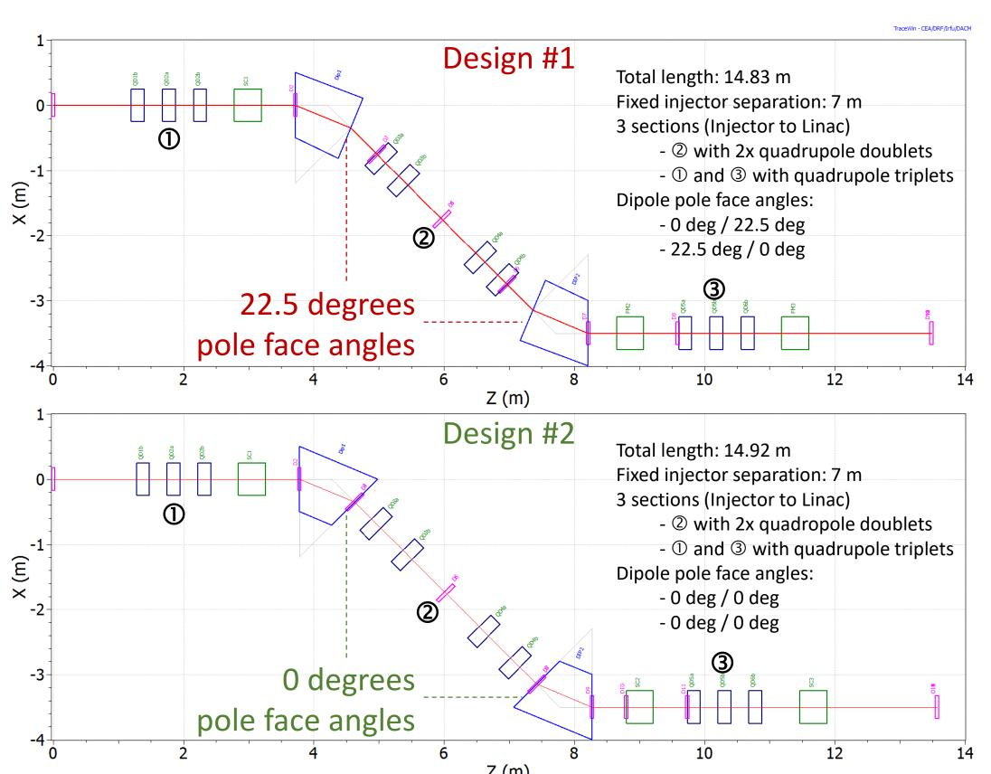
Two alternative designs of the MEBT-3 lattice are shown. Design #1 (top) uses 22.5° for the pole face angles in section ②, whereas Design #2 (bottom) has straight pole faces.
