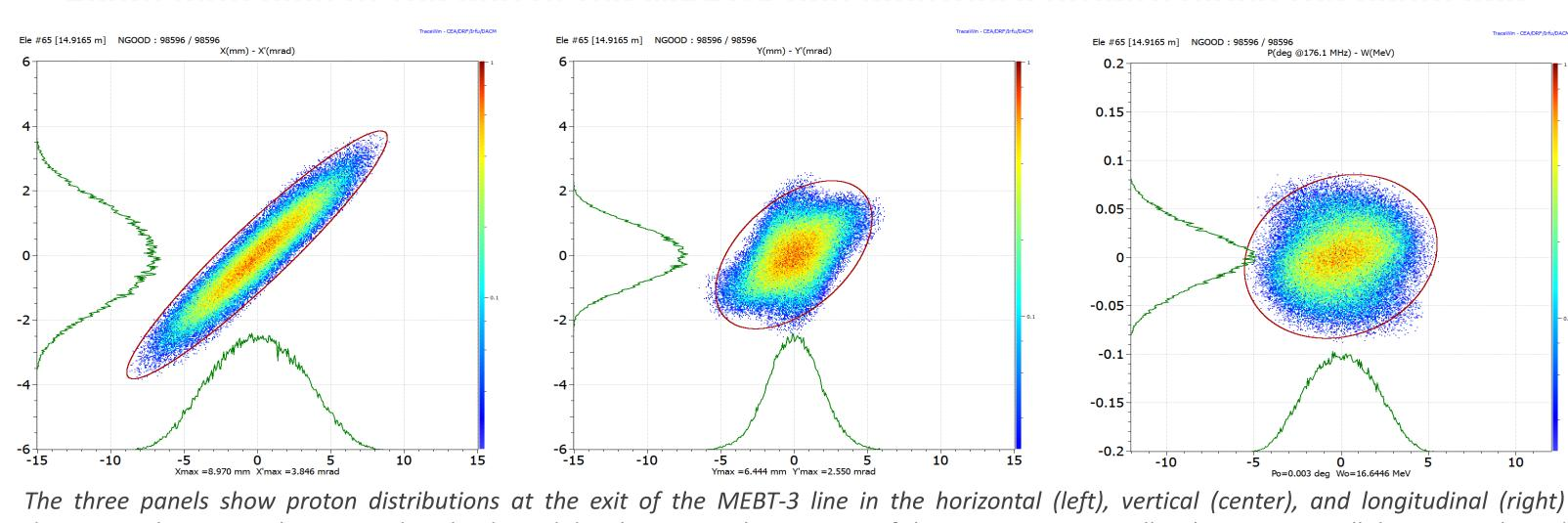
The three panels show proton distributions at the exit of the MEBT-3 line in the horizontal (left), vertical (center), and longitudinal (right) directions. The mismatch compared to the desired distributions at the entrance of the main LINAC is smaller than 0.12% in all directions. The red ellipses correspond to an emittance of 9 rms.
