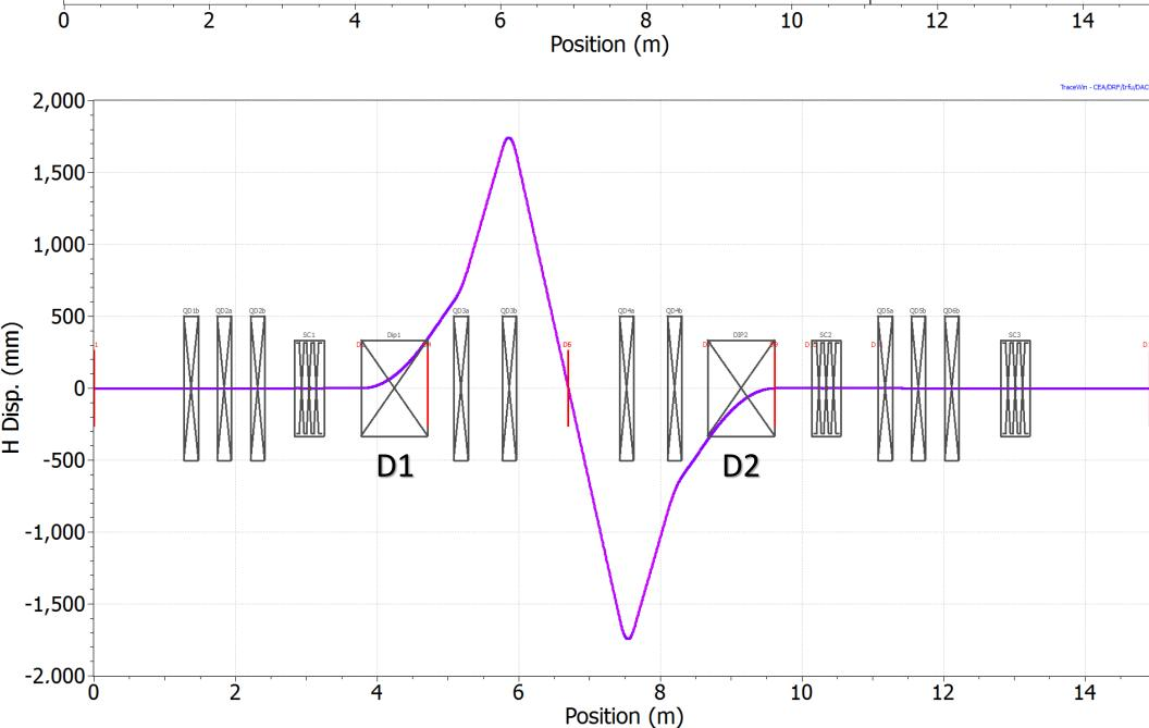
The top panel shows  $\pm 3\sigma$  envelopes in the two transverse directions (purple - horizontal plane, green - vertical). The bottom is showing the dispersion being compensated after the switching dipole and satisfying the double achromaticity condition.
