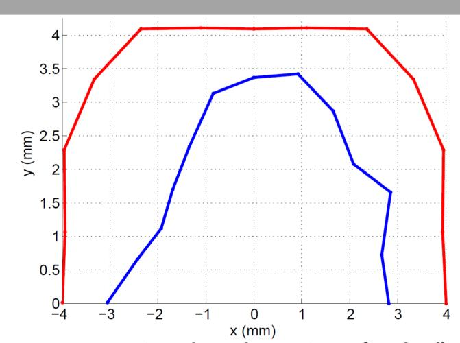
Transverse on-momentum dynamic aperture of a -I cell, with natural chromaticities. In red, the lattice without RF, in blue, RF system added, with a voltage of 1.1 MV.
