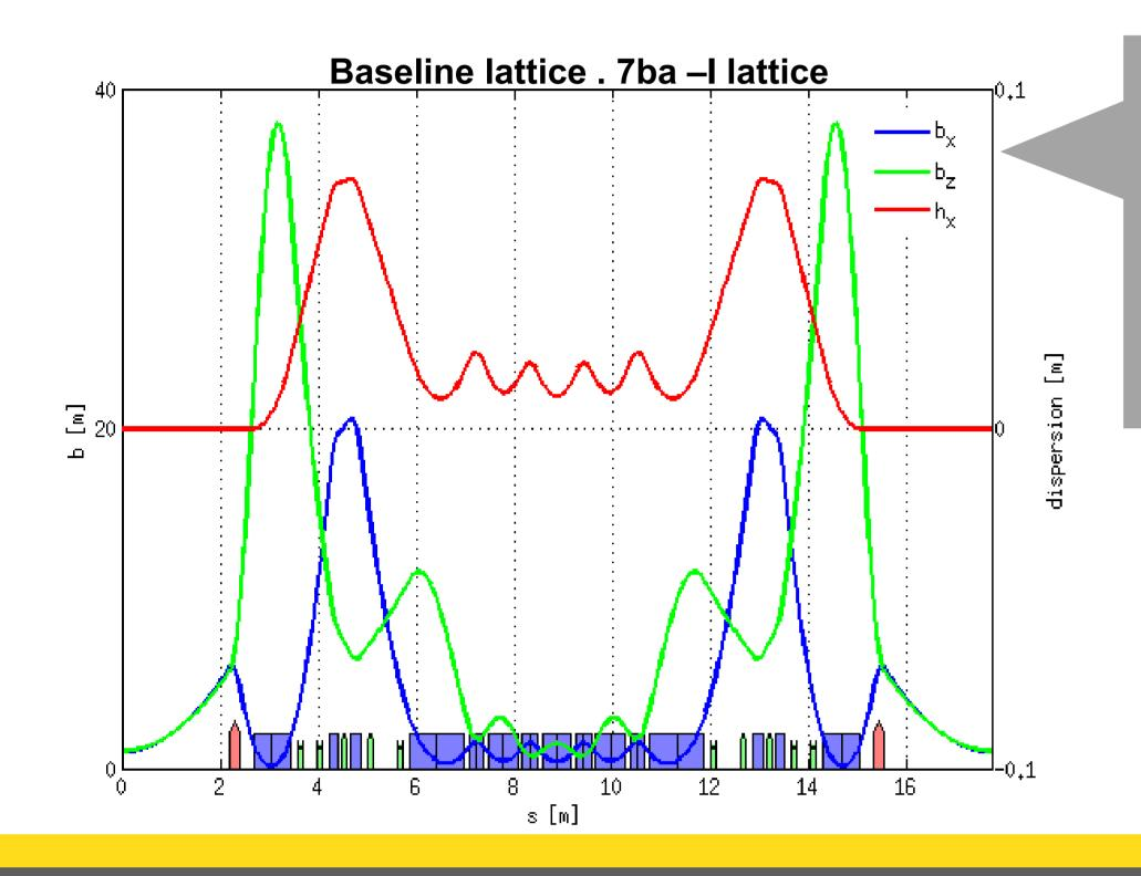
The baseline lattice uses the \$-I\$ transformation, setting  $a((2k+1)\pi, n\pi)$  phase advance between two sextupoles (with  $k, n \in \mathbb{N}$ ) for:
