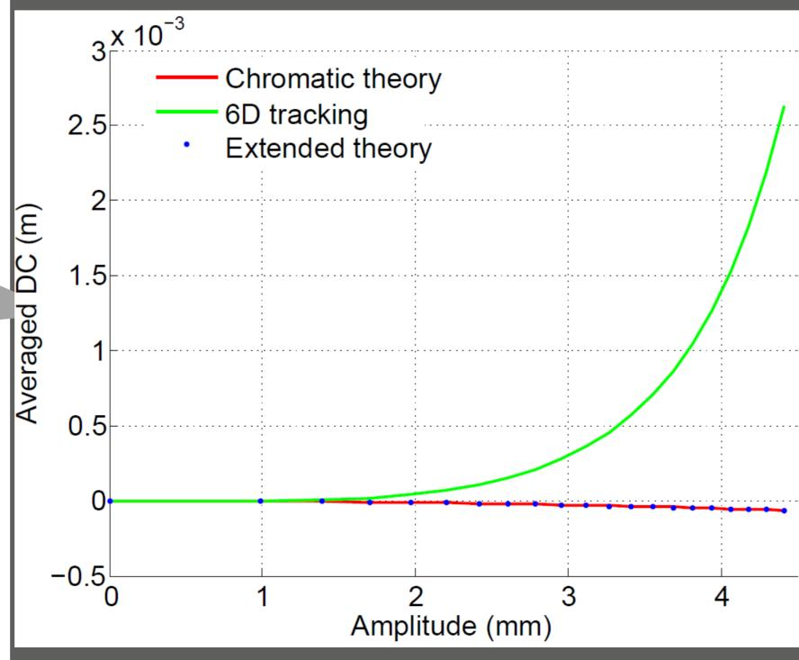
Averaged path lengthening considering the three described methods -- linear formula of  $\Delta C$  in red, 6D tracking of the -/ lattice in green and perturbed path length using the distorted trajectory on the side, for
