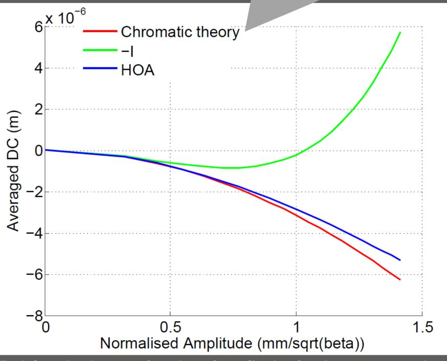
Path lengthening as a function of amplitude after 1 turn, averaged on the input phase, for both -I and HOA lattices, at a corrected chromaticity of (1,1).
