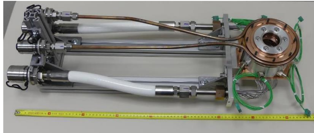
Target + collimator + water cooling + T measurement
