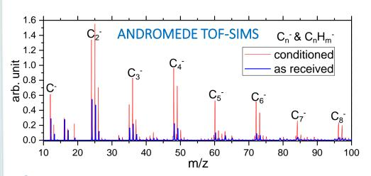
(5) Conditioning effect and graphitization: Beam pipe surface chemistry is modified by interactions with electrons (EC).
