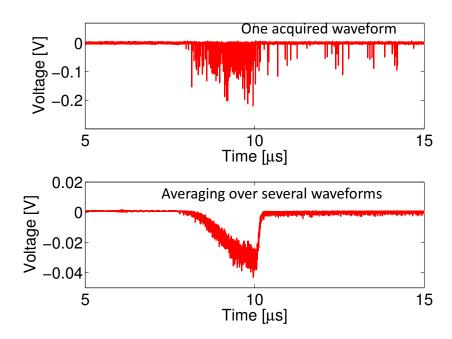
The measured position accuracy allows resolving the beam losses occurring as close as 30 - 40 cm with the 25 m fiber along the vacuum chamber.
